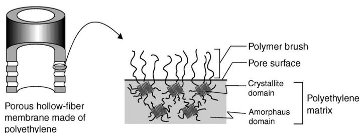
Fig. 1. Definitions for polymer brushes grafted onto the pore surface of a porous hollow-fiber membrane.
