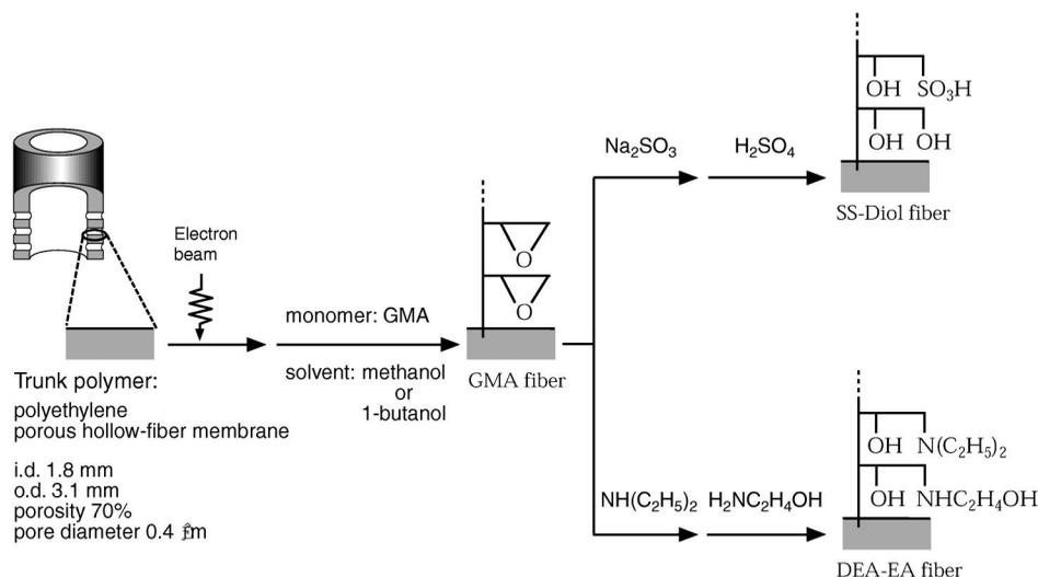
Fig. 2. Introduction of two charged groups into the polymer brush.
