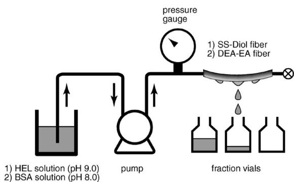
Fig. 3. Experimental apparatus for protein binding during permeation of protein solution.
