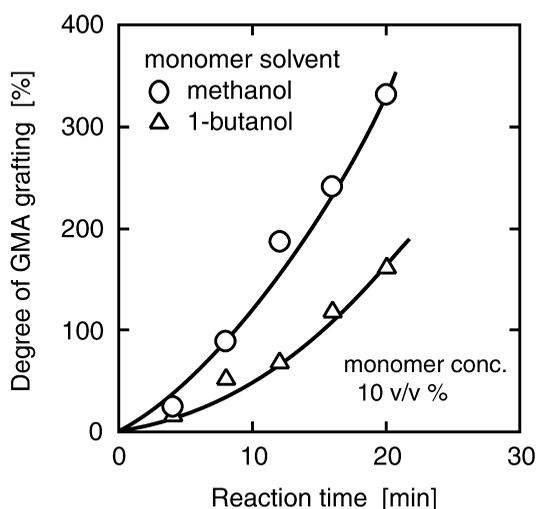
Fig. 4. Grafting rate of glycidyl methacrylate.
